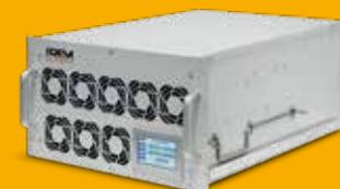
The IREM active harmonic filter AHF series implements a process of compensation of the harmonic content: the harmonic current produced by the load is constantly monitored and an adaptive waveform is generated, that corresponds to the exact shape of the non-linear portion of the load current. The AHF introduces this adaptive current into the load at the connection point with a reaction time of 50  $\mu$ s and a response time of 5ms.
